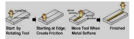
Figure 1: shows the schematic flow process of friction stir welding
