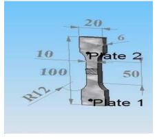
Figure 5: Design for tensile specimen
