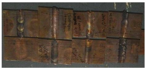
**Figure 3: friction stir weld samples**
