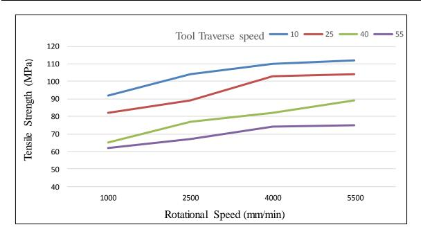
Figure 7: Tensile behaviour of FSW joints for varying rotational speed with different travel speed
