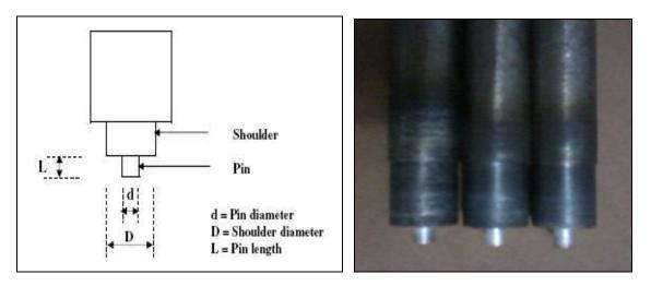
Figure 2(A and B): A- drawing for FSW tool; B- tool prepared for FSW
